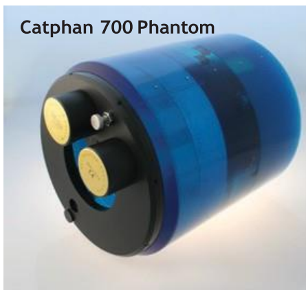
Figure 7a. Catphan 700 Phantom Includes Low-Contrast Module with Different Supra-Slice and Subslice Contrast Targets
